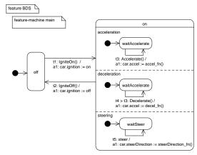
Fig. 1. Basic Driving Service (BDS) standalone feature machine
