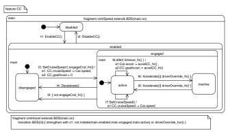
Fig. 2. Cruise Control (CC) feature-machine fragments
